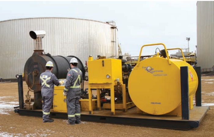
8,000,000 BTU/hr Fired Heating Unit
