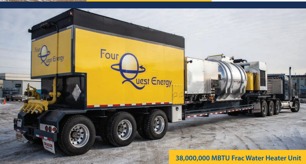
8,000,000 BTU/hr Fired Heating Unit
